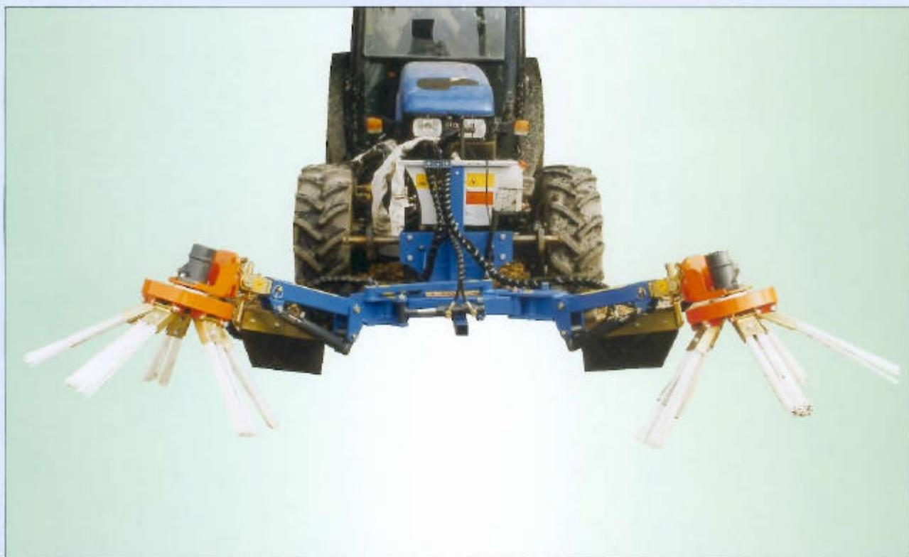
ANDANATORE ANTERIORE CON DUE TESTATE INDIPENDENTI, SERVOASSISTITO DA ELETTROVALVOLE E CENTRALINA ELETTRICA
